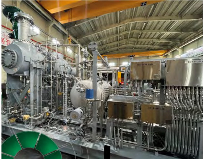
The Rotoflow EC 40 turboexpander is available in two types: oil-bearing or mag-bearing. Rotoflow's high-pressure compressor-loaded turboexpanders (componders) provide refrigeration for the most efficient air separation and liquefaction facilities in the world. Credit: Rotoflow.
